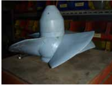
Propeller S-Turbine head: 2 – 13 meter power: 10 - 150 kW
