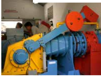
X-flow Turbine T-14 D300 head: 3 – 100 meter power: 10 – 150 kW
