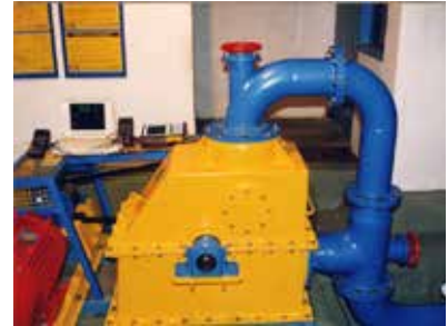
Pelton Turbine head: 70 – 300 meter power: 50 – 1000 kW
