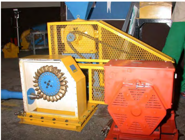
Peltric Turbine head: 15 – 100 meter power: 1 – 30 kW
