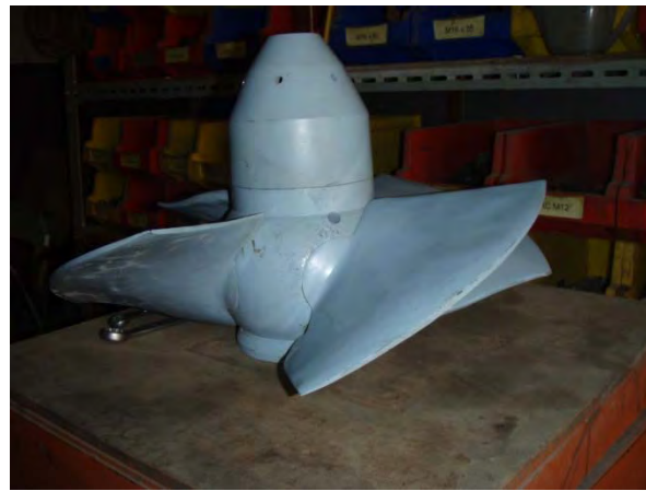
Propeller S-Turbine head: 2 – 13 meter power: 10 - 150 kW
