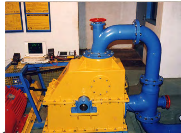
Pelton Turbine head: 70 – 300 meter power: 50 – 1000 kW
