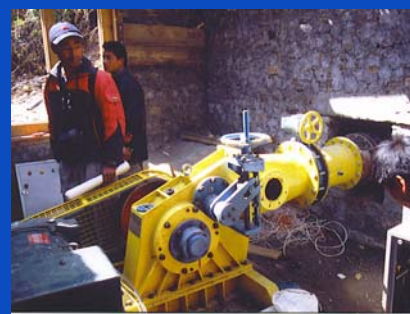
Basa Khola, Solokhumbu, Nepal X-flow T-14, ELC-40 kW 2004
