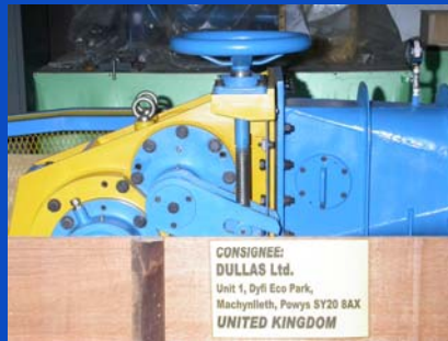
Alwen WTW, Wales, UK X-flow T-14, IMAG-25 kW 2006
